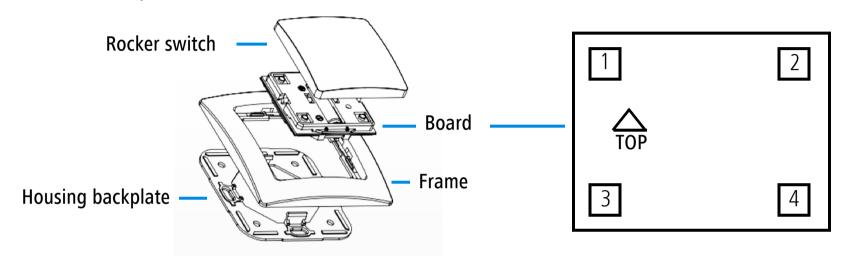
4 If you fasten the Home Control Wall Switch using the double-sided tape for corners, put this tape on the four corners of the housing backplate and attach the Home Control Wall Switch to the place you want it to be.
