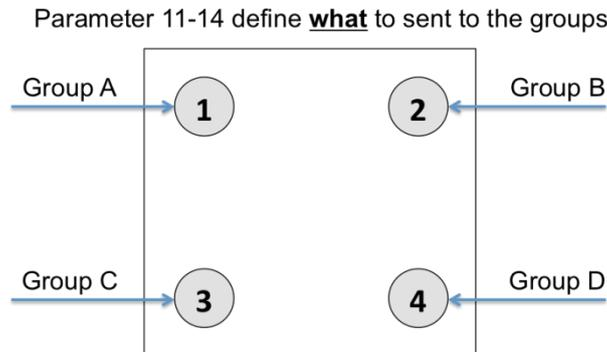
**2 Groups are controlled with two buttons (parameter 1 or 2 => 1)** The buttons 1 and 3 control the control group A (button on turns on, buttons turns off), the buttons 2 and 4 control the control group B (button on turns on, buttons turns off). In case dimmers are controlled, holding down the larger button will dim up, holding down the smaller button will dim down the load. Releasing the button will stop the dimming function.
