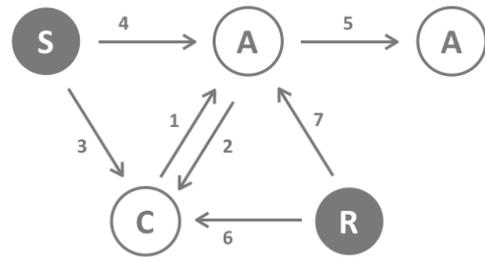
There are two different roles a controller can have. There is always one single primary controller that is managing the network and including/excluding devices. The controller may have other functions - like control buttons - as well. All other controllers don't manage the network itself but can control other devices. They are called secondary controllers. The image also shows that its not possible to operate a sensor just from a remote control. Sensors only communicate with static controllers.
