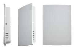
5430128 **EXTERNAL ROOM SENSOR** External room sensor with glass front face. Wall mounted. NTC 10 kOhm Size: (LxWxH) 80x110mmx16mm
