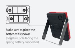
Power on the device Slide the power switch
