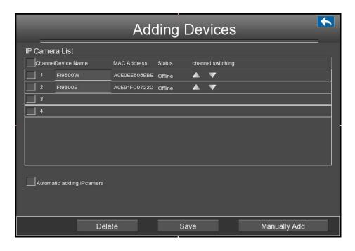
NVR will automatically detect all the online IP Cameras which they can connect to. You will need to know your IP Camera name and password to connect.
