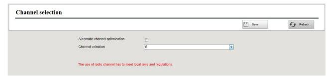
The default selection is Automatic channel optimization, NVR chooses the channel automatic. Or you can select the channel from the dropdown list. Don't tick Automatic channel optimization when you want to select the channel manually.
