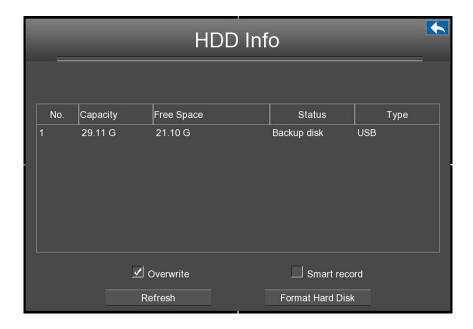
**Overwrite**: When the HDD is full. You check the **Overwrite** checkbox, the NVR will cycle cover the earliest recording; If not, the NVR will stop recording when the HDD is full.
