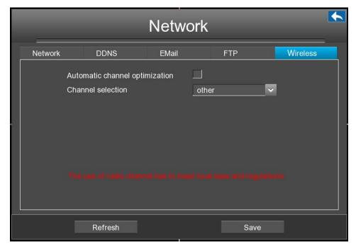
Select **Automatic Channel Optimization**, NVR will choose the channel automatic. Or you can select the channel from the dropdown list. Don't tick **Automatic channel optimization** when you want to select the channel manually.
