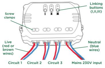
**IMPORTANT:** Max. output (total of three circuits) 3000W.
