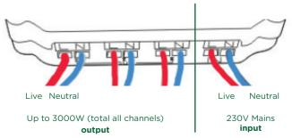
The 3-Way Relay requires mains power to operate. It can be used to provide mains power to and switch on/off three separate 230V circuits independently. The relay can provide a maximum of 3000W in **total** across the three circuits (not 3000W **per** circuit).
