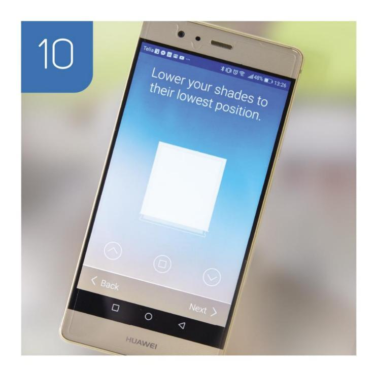
Start the configuration process. Set high and low points for the blinds.
