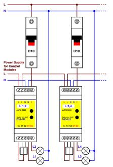
The descriptions of the screw terminals are printed on the adapter label. The letter "I" indicates input for powering the load devices. The "Q1" and "Q2" letters indicate the relays outputs.
