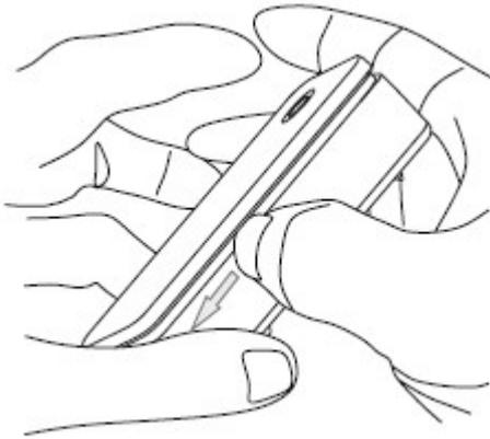
3. Once the battery cover is separated from the Sensor Unit, you can pull out and change the battery located in the center of the Water Sensor 6 hardware.
