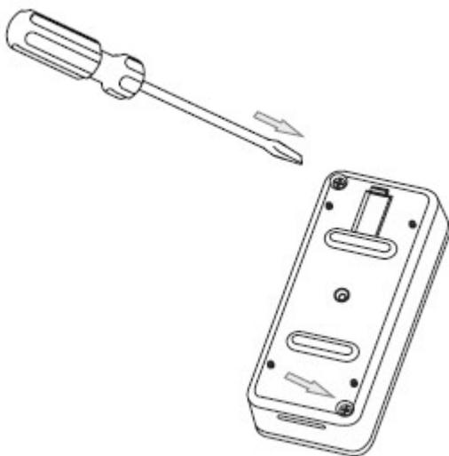
2. Separate the battery cover from the Sensor unit. Use the separation tool to separate the battery cover by pushing or moving the separation along the gap between the battery cover and the sensor unit.
