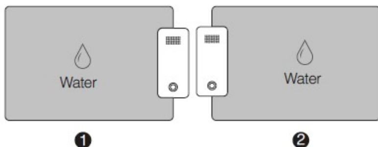
3. Water is detected by sensing point 1 and 2.
