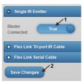
To use the Blaster cable with the Flex Link Tri-port cable, plug it into the port labeled IR3, select "Flex Link Tri-port Cable," and select **True** for the **Blaster Connected on IR3** setting. **Save Changes** to apply new settings.
