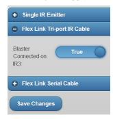
Please note the Blaster cable is designed to be used with Global Caché iTach Flex products to transmit IR signals across a room up to 35 feet. The IR modulation frequency 20 to 500 KHz
