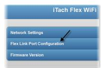
The 3 IR ports on the Tri-port cable can be used as 3 IR emitters (same as the 3 Emitter cable) or 2 emitters and 1 Flex Link Blaster cable on IR3, similar to the 2E1B cable. To use the 2E1B cable or IR3 with a Flex Link Blaster cable, change "Blaster Connected on IR3" from False to **True**. Then select **Save Changes** to apply the new settings.
