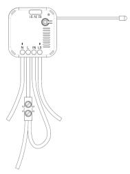
**Note:** Please use 1.25m m<sup>2</sup> wires. When there are two or more wires, please use the appropriate external terminal wiring as shown above.
