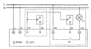
As illustrated in the above diagram, S1 provides a wall switch connection to the dry contacts. By default S1 switch supports Single-Pole-Double-Throw (SPDT) type of binary switch. However, through the setting of Gateway, S1 can be configured to support Toggle switches as well. The S2 switch can also switch the on/off status of the unit when toggled.
